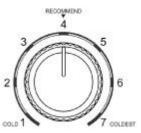
3. It is recommended to adjust the air regulating rod in the middle position. When the user needs a lower freezer temperature, adjust the air regulating rod to the right properly, then the freezer temperature decreases while the fridge temperature rises. When the temperature meets the requirement, adjust the air regulating rod back to the middle position again in a timely manner.
