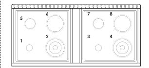
BURNER 1 SMALL (6,000 BTU) BURNER 2 DUAL (20,000 BTU) BURNER 3 SMALL (6,000 BTU) BURNER 4 DUAL (20,000 BTU) BURNER 5 STRD (9,000 BTU) BURNER 6 LARGE (12,000 BTU) BURNER 7 STRD (9,000 BTU) BURNER 8 LARGE (12,000 BTU)
