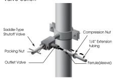
4. Flush the tubing. Turn the main water supply on and flush out the tubing until the water is clear. Then, shut the water off at the water valve after about a quart of water has flushed through the tubing.
