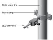
Connect 1/4" extension tubing to shutoff valve outlet.
